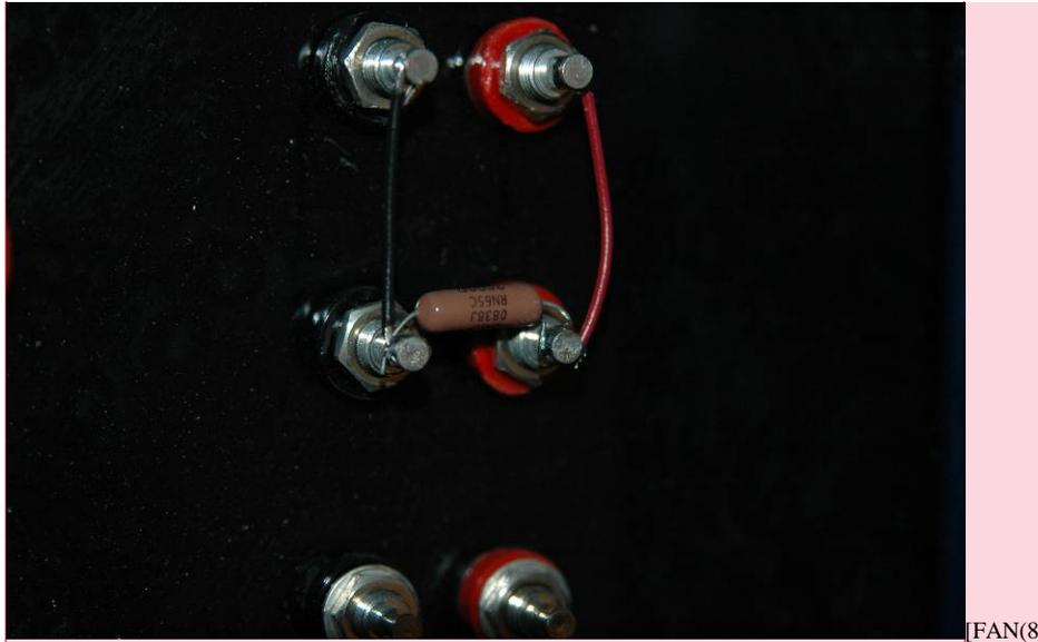
Figure 8. 250 ohm resistors used in patch panels
