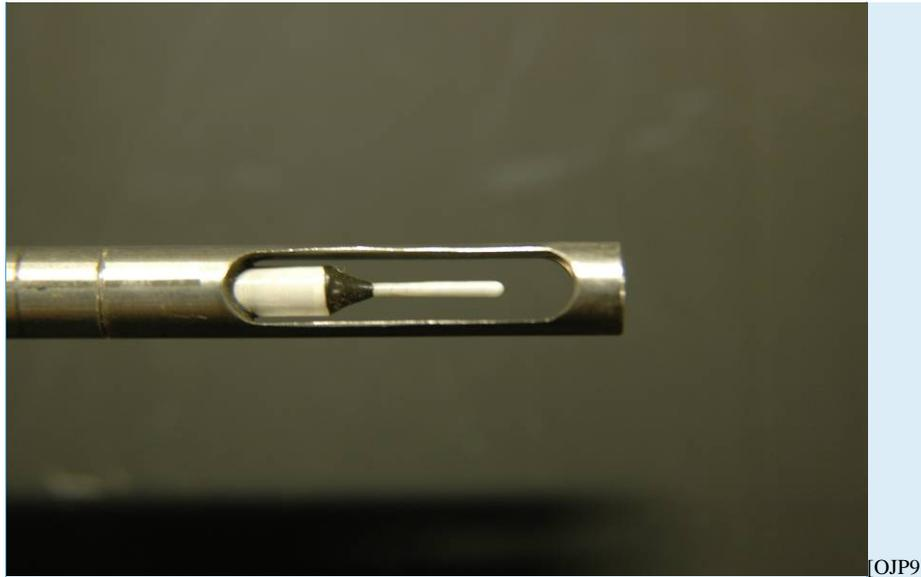
Figure 9. Hot wire sensor
