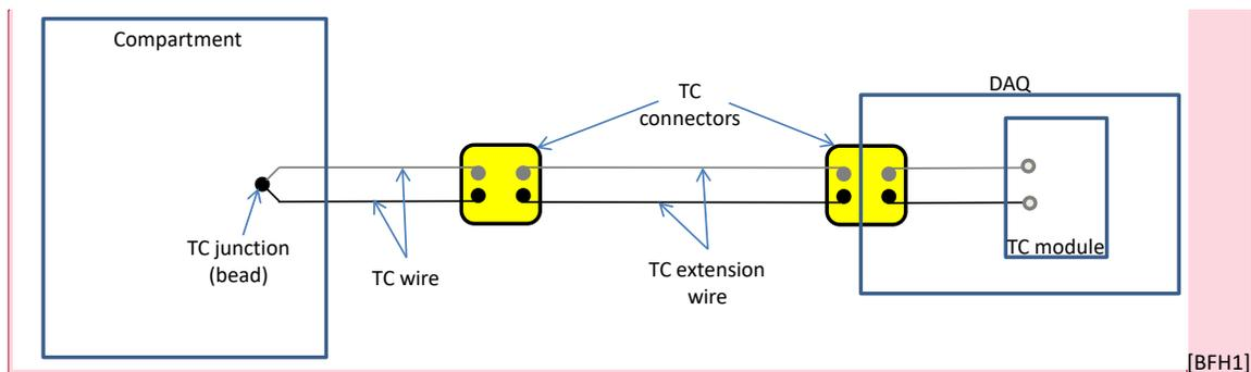
Figure 1. Thermocouple measurement system
