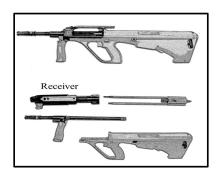
(vii) Thompson M1A1-type machineguns and semiautomatic variants, and L1A1, FN FAL, FN FNC, MP38, MP 40, and SIG 550-type firearms, and HK-type machineguns and semiautomatic variants: the upper part of the weapon that provides housing for the bolt and firing pin.
