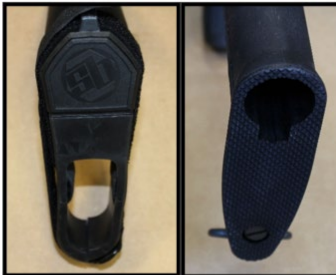
Surface area of SBA3 “stabilizing brace” (left) compared to known AR-15 stock (right)
