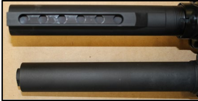
Adjustable Rifle Buffer Tube (top) compared to a Standard Pistol Receiver Extension (bottom)
