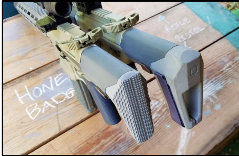
The Q Honey Badger Rifle with a stock (left) and the Q Honey Badger Pistol with a “stabilizing brace” (right) 118
