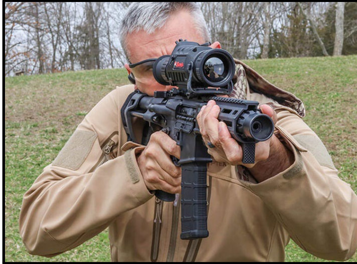
Example of firearm with thermal scope with eye relief that requires shouldering of the firearm in order to be used as designed.
