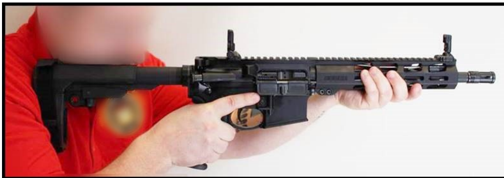
The use of a rifle receiver extension provides horizontal support for use as a shouldering device.
