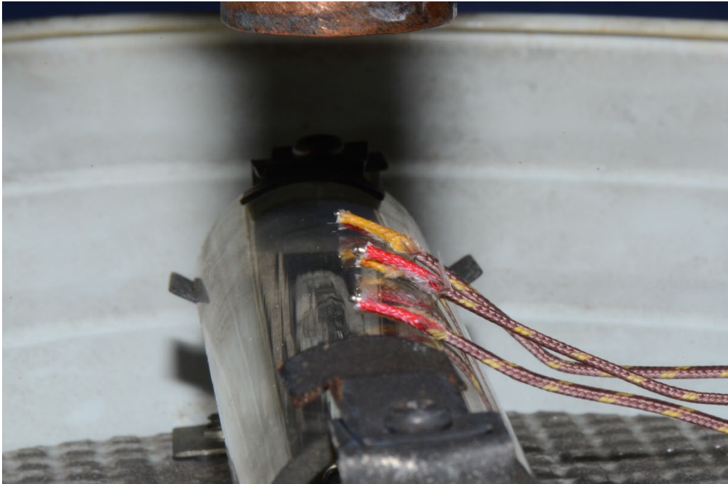
Figure 6: Thermocouples placed on top of the protective shield, in line with the center of the lamp. (61654_543389)
