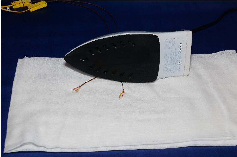
Figure 2. Placement of thermocouples. 51309_515188.jpg
