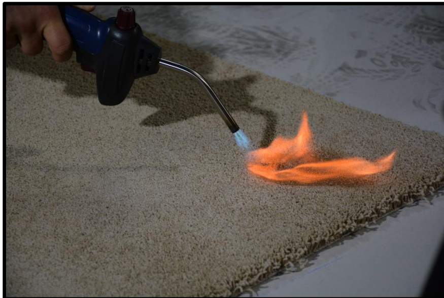
Figure 17. Torch flame applied to carpet surface (193896_793422.jpg)
