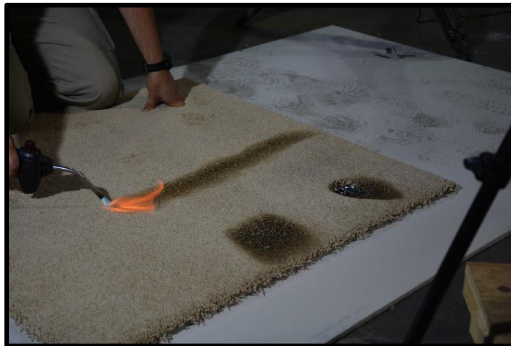
Figure 14. Propane Torch Applied to Carpet Surface (193896_793443.jpg)
