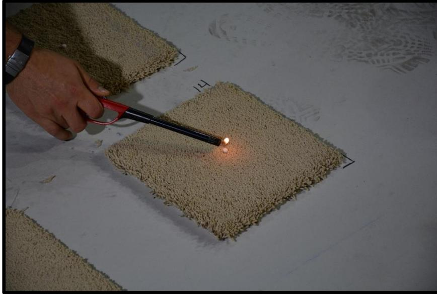
**Figure 4. Ignition of methenamine pill (203912\_804059.jpg)**
