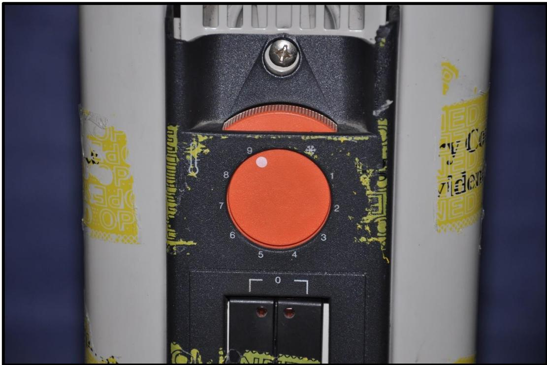
**Figure 3. Rotary Thermostat Switch (284707\_993841.jpg)**
