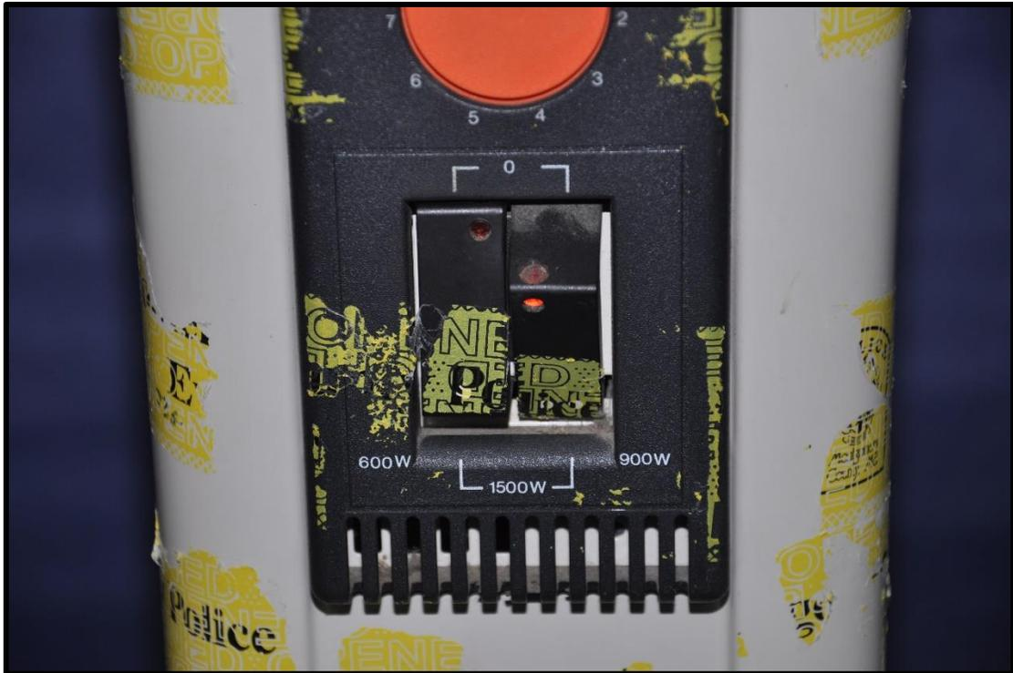
**Figure 2. Adjustable Wattage Toggle Switch (284707\_993846.jpg)**
