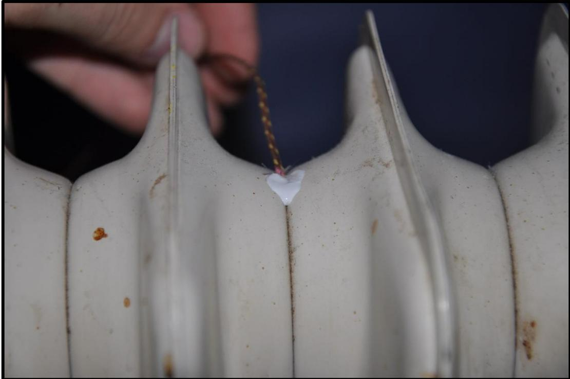
**Figure 6. Thermocouple - Thermal Paste Interface (284707\_994361.jpg)**
