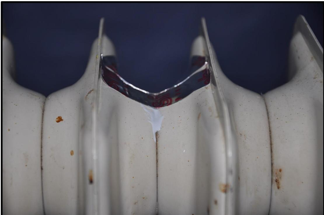
**Figure 7. Taped Thermocouple (284707\_994362.jpg)**
