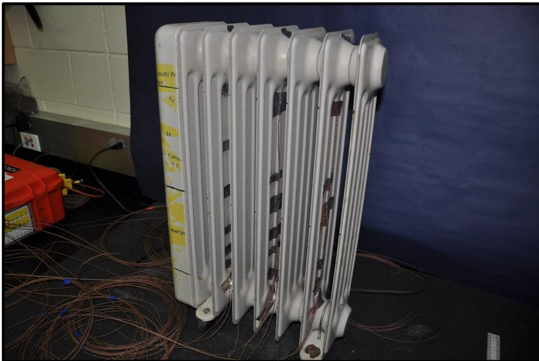
**Figure 9. Thermocouples Attached to Heater (284707\_994431.jpg)**
