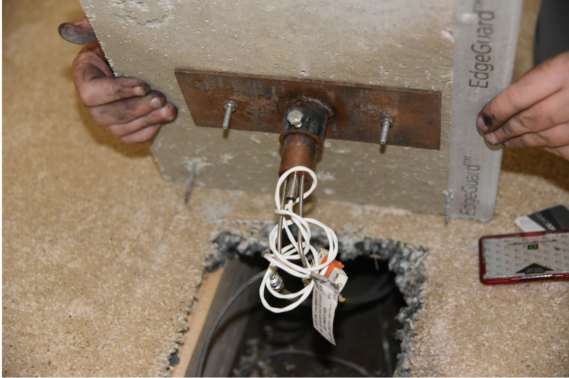
Figure 4. Hole in floor to accommodate heat flux transducer mounted to the bottom of the cement board (337704_1190298.jpg)
