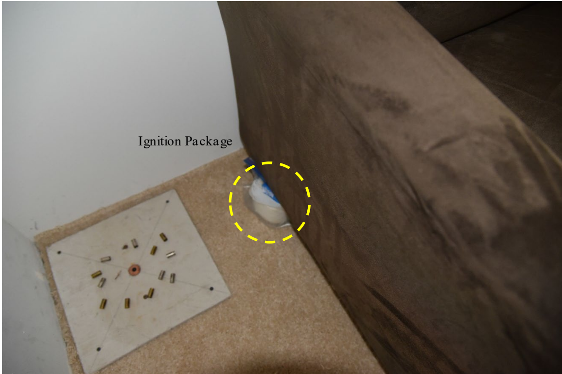
Figure 8. Ignition package located under left rear corner of sofa (337704_1190348.jpg)
