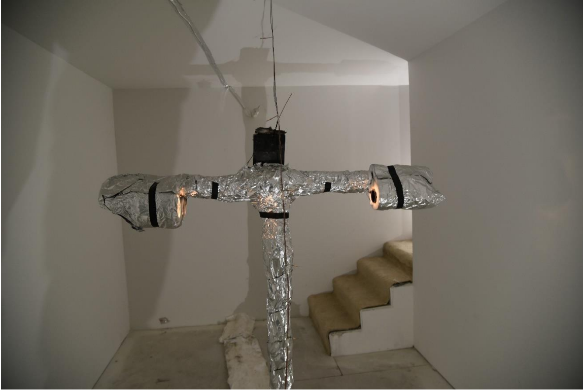
Figure 21. Instrumentation stand for tenability measurements (360086_1305132.jpg)
