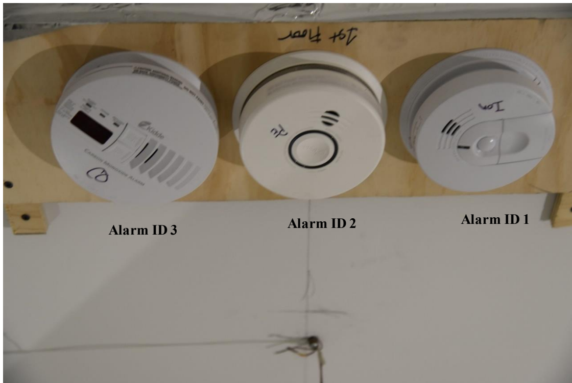
Figure 16. AC powered alarms – image annotated (360079_1304666.jpg)
