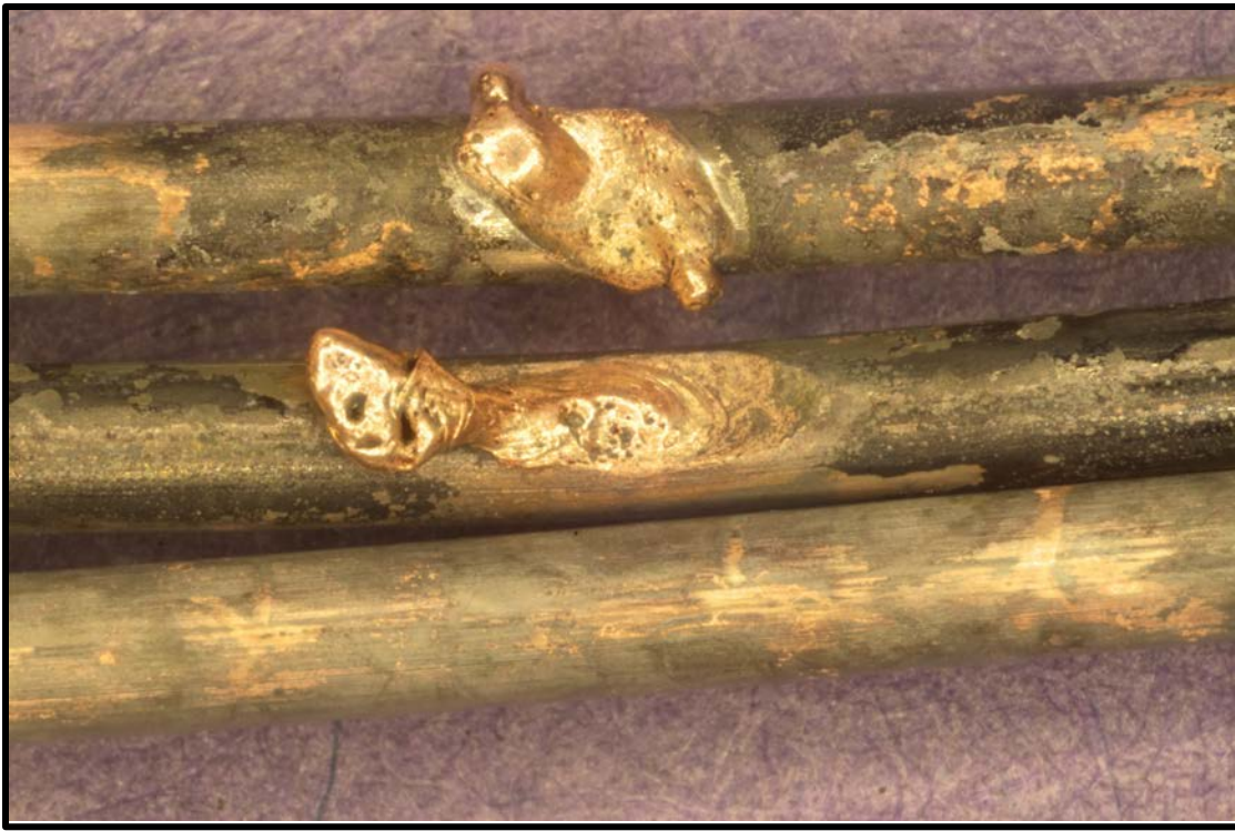
Figure 1. Arc melting produced in Test 1 of an AFCI circuit breaker at 35 kW/m 2 .
