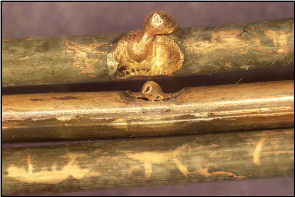
Figure 43. Arc melting produced during Test 2 of a TM circuit breaker at 35 \text{ kW/m}^2 .
