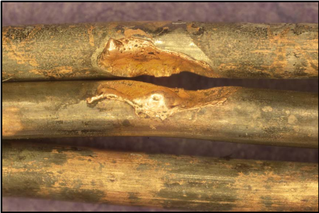
Figure 45. Arc melting produced during Test 3 of a TM circuit breaker at 35 \text{ kW/m}^2 .
