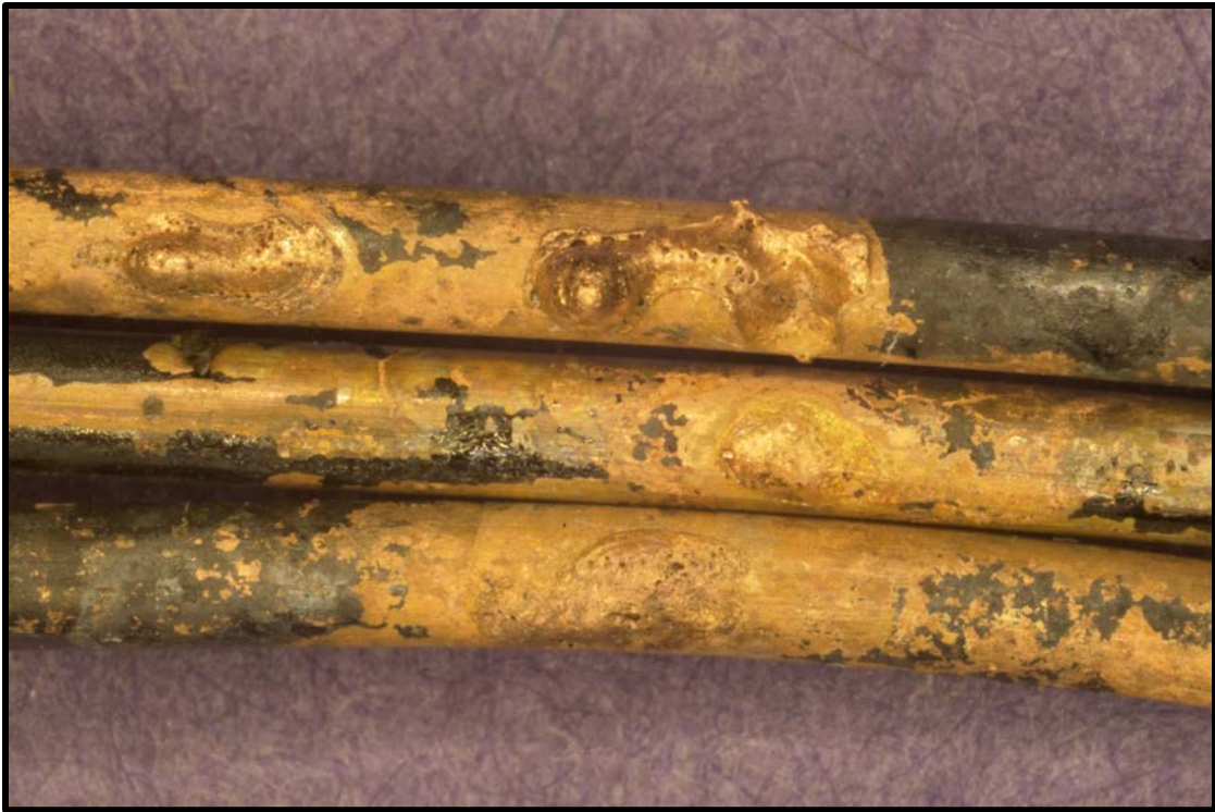
Figure 57. Arc melting produced during Test 3 of a TM circuit breaker at 55 \text{ kW/m}^2 .
