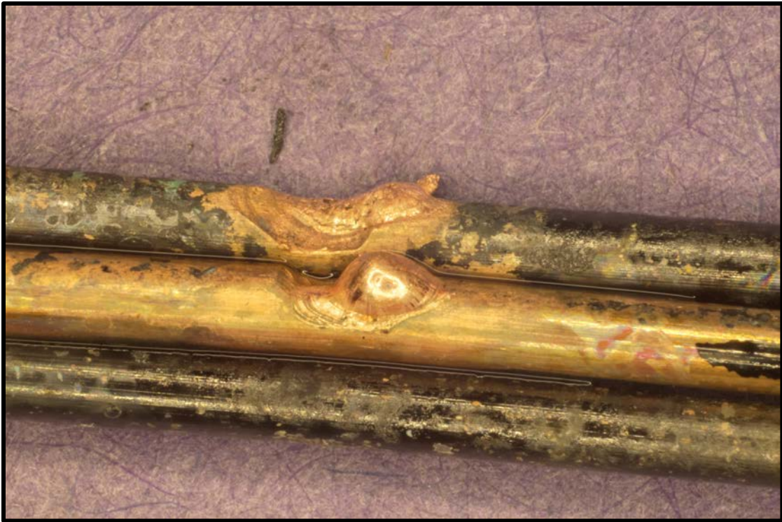
Figure 13. Arc melting produced during Test 4 of an AFCI circuit breaker at 45 kW/m 2 .
