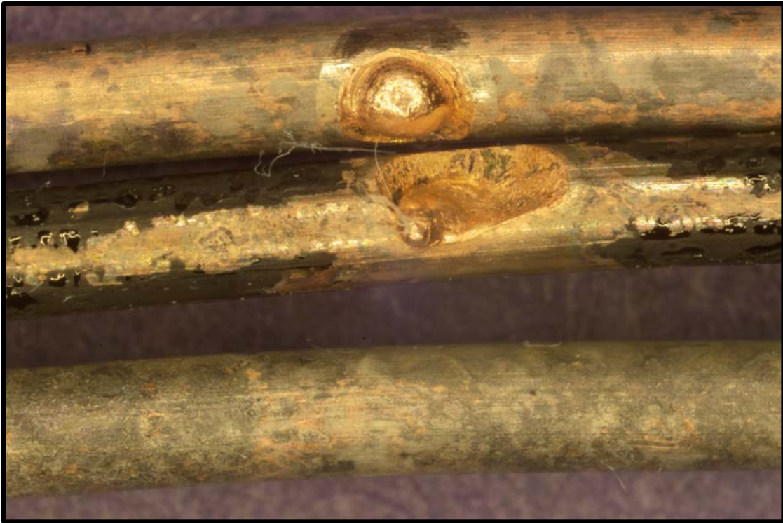
Figure 47. Arc melting produced during Test 1 of a TM circuit breaker at 45 \text{ kW/m}^2 .
