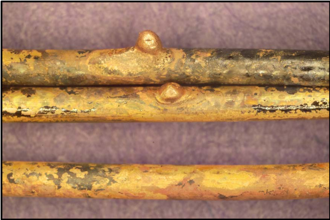
Figure 39. Arc melting produced during Test 3 of a GFCI circuit breaker at 55 kW/m 2 .
