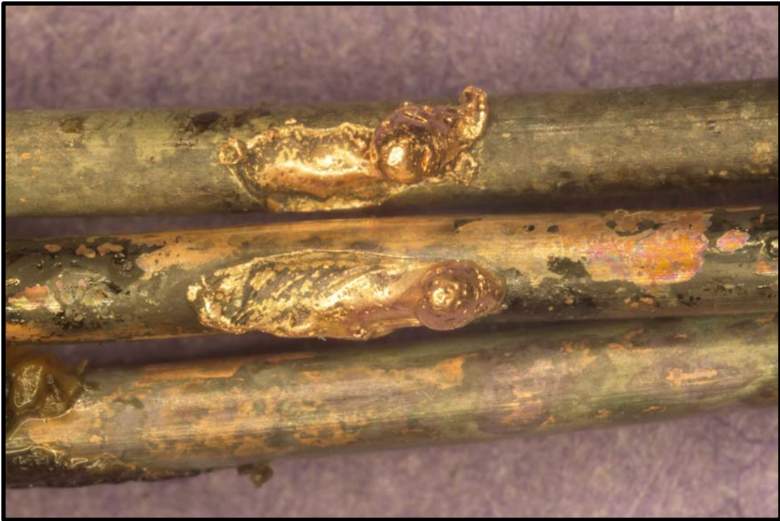
Figure 55. Arc melting produced during Test 2 of a TM circuit breaker at 55 \text{ kW/m}^2 .
