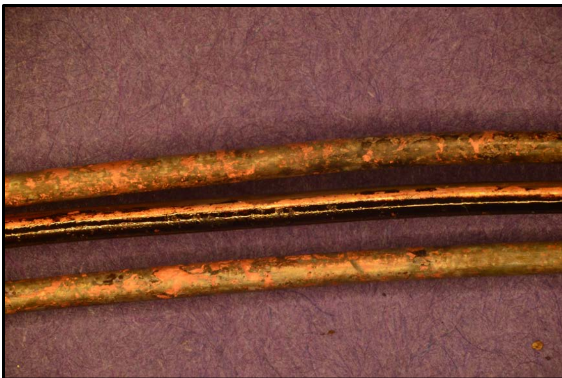
Figure 37. Absence of arc melting produced during Test 2 of a GFCI circuit breaker at 55 kW/m 2 .
