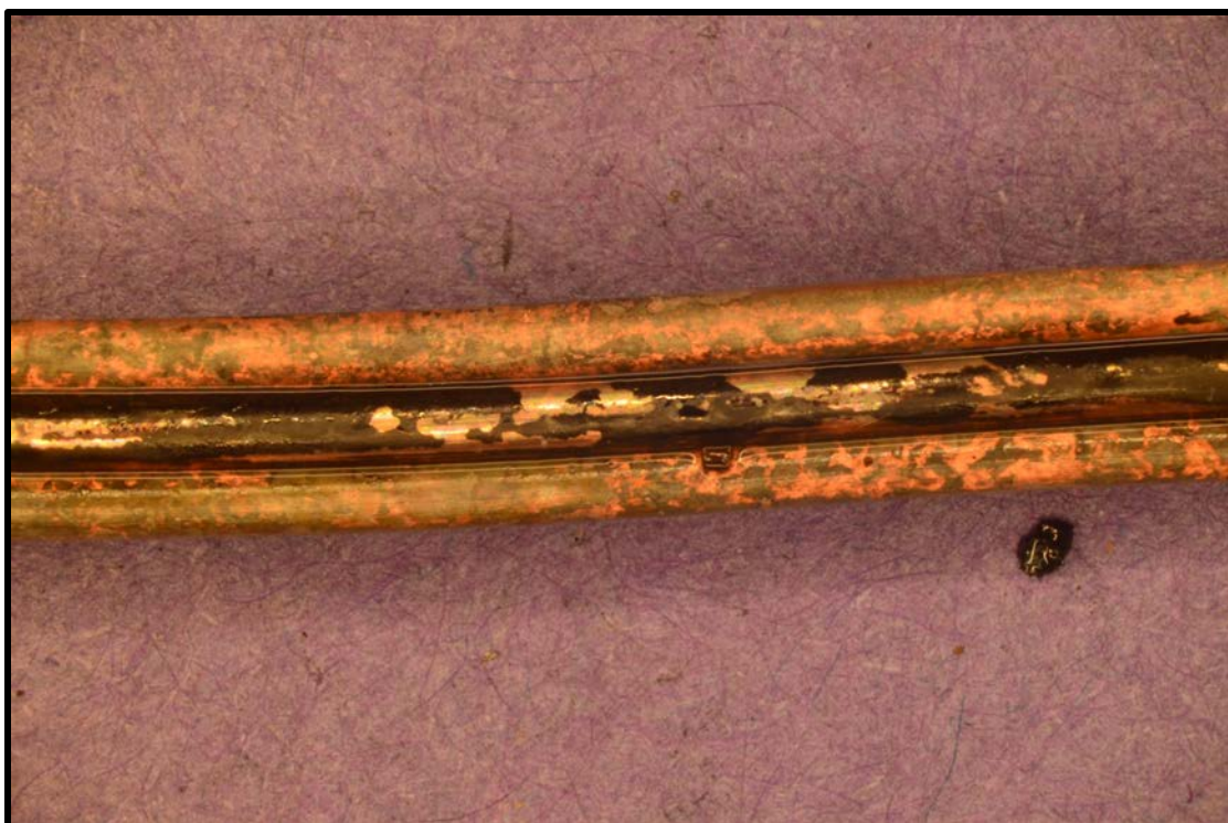
Figure 11. Absence of arc melting produced during Test 3 of an AFCI circuit breaker at 45 kW/m 2 .
