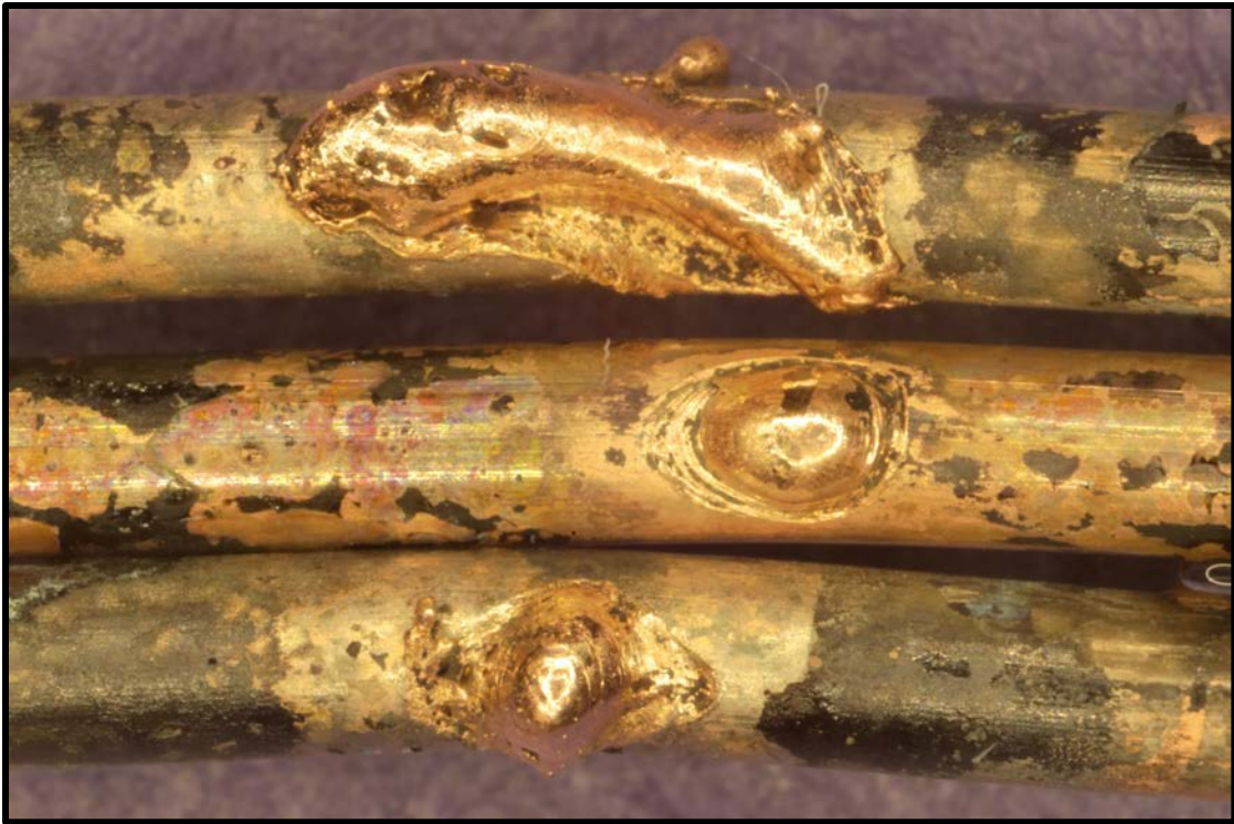
Figure 53. Arc melting produced during Test 1 of a TM circuit breaker at 55 \text{ kW/m}^2 .
