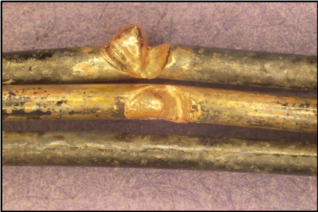
Figure 17. Arc melting produced during Test 2 of an AFCI circuit breaker at 55 kW/m 2 .
