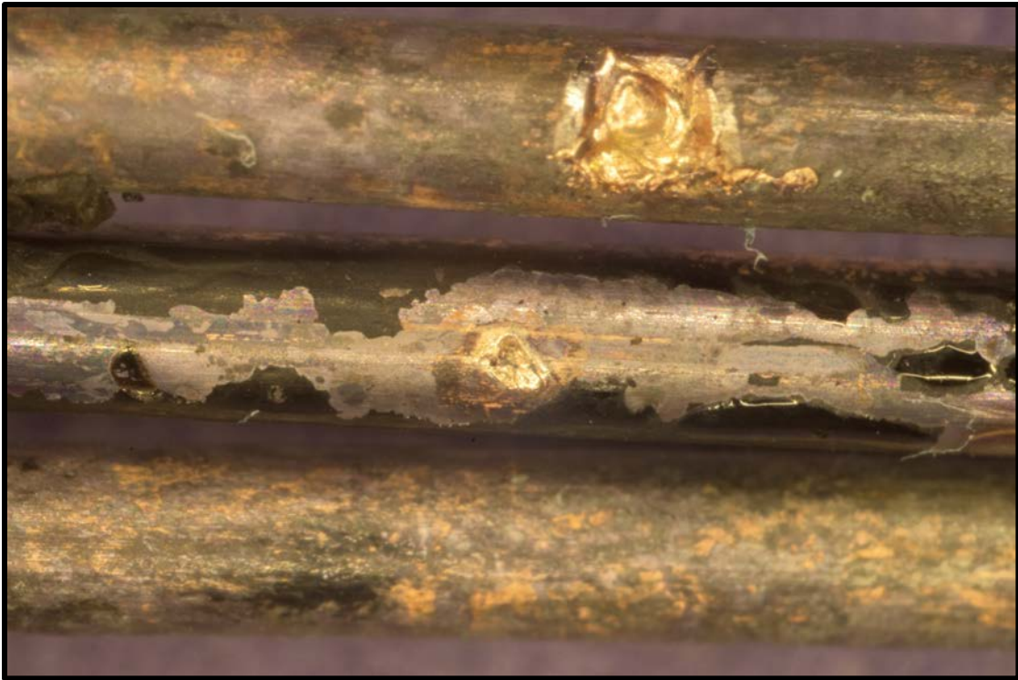
Figure 49. Arc melting produced during Test 2 of a TM circuit breaker at 45 kW/m 2 .
