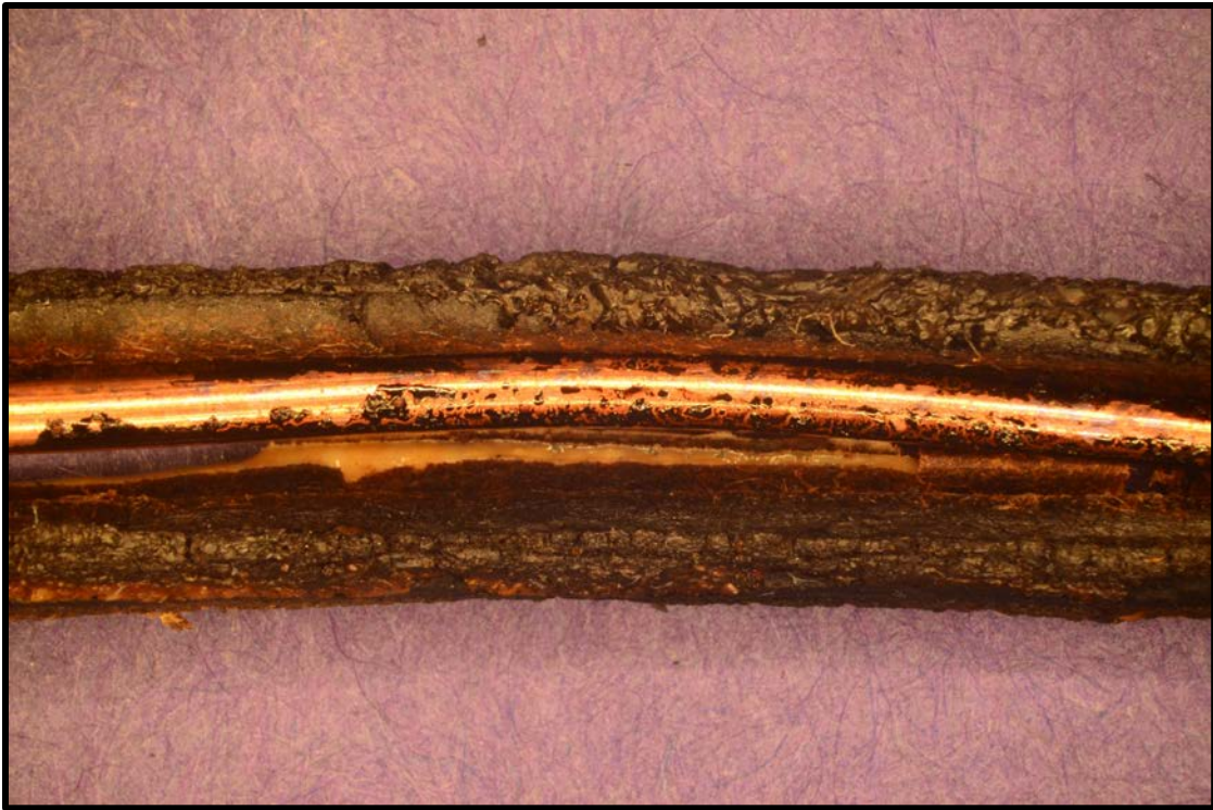
Figure 35. Absence of arc melting produced during Test 1 of a GFCI circuit breaker at 55 kW/m 2 .
