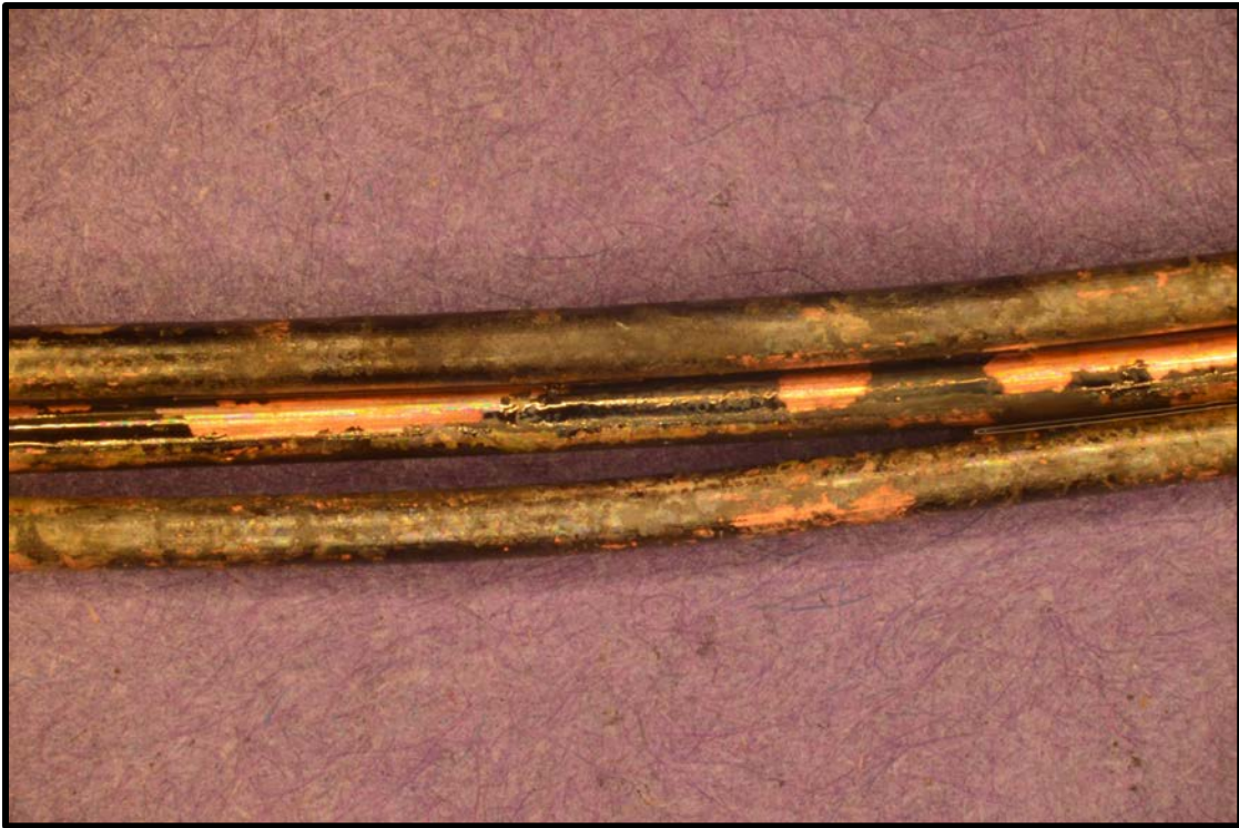
Figure 9. Absence of arc melting produced during Test 2 of an AFCI circuit breaker at 45 kW/m 2 .
