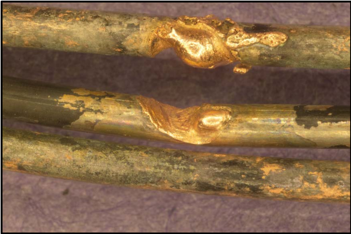
Figure 25. Arc melting produced during Test 3 of a GFCI circuit breaker at 35 kW/m 2 .
