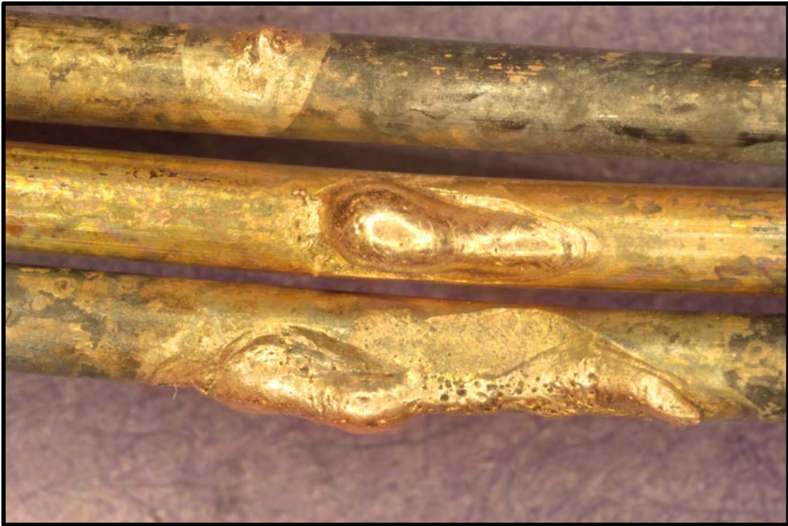
Figure 19. Arc melting produced during Test 3 of an AFCI circuit breaker at 55 kW/m 2 .
