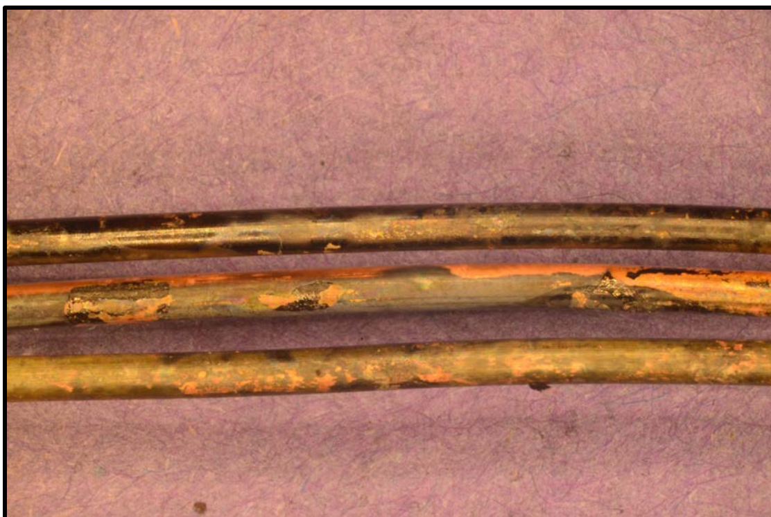
Figure 7. Absence of arc melting produced during Test 1 of an AFCI circuit breaker at 45 kW/m 2 .
