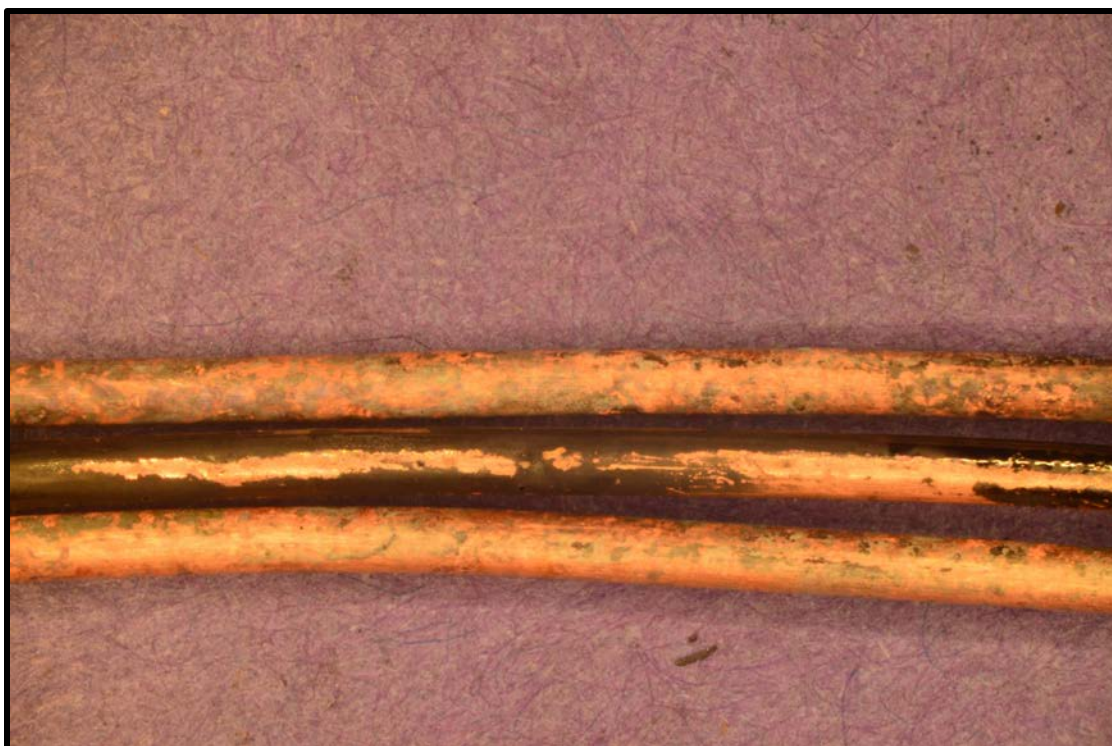
Figure 23. Absence of arc melting produced during Test 2 of a GFCI circuit breaker at 35 kW/m 2 .
