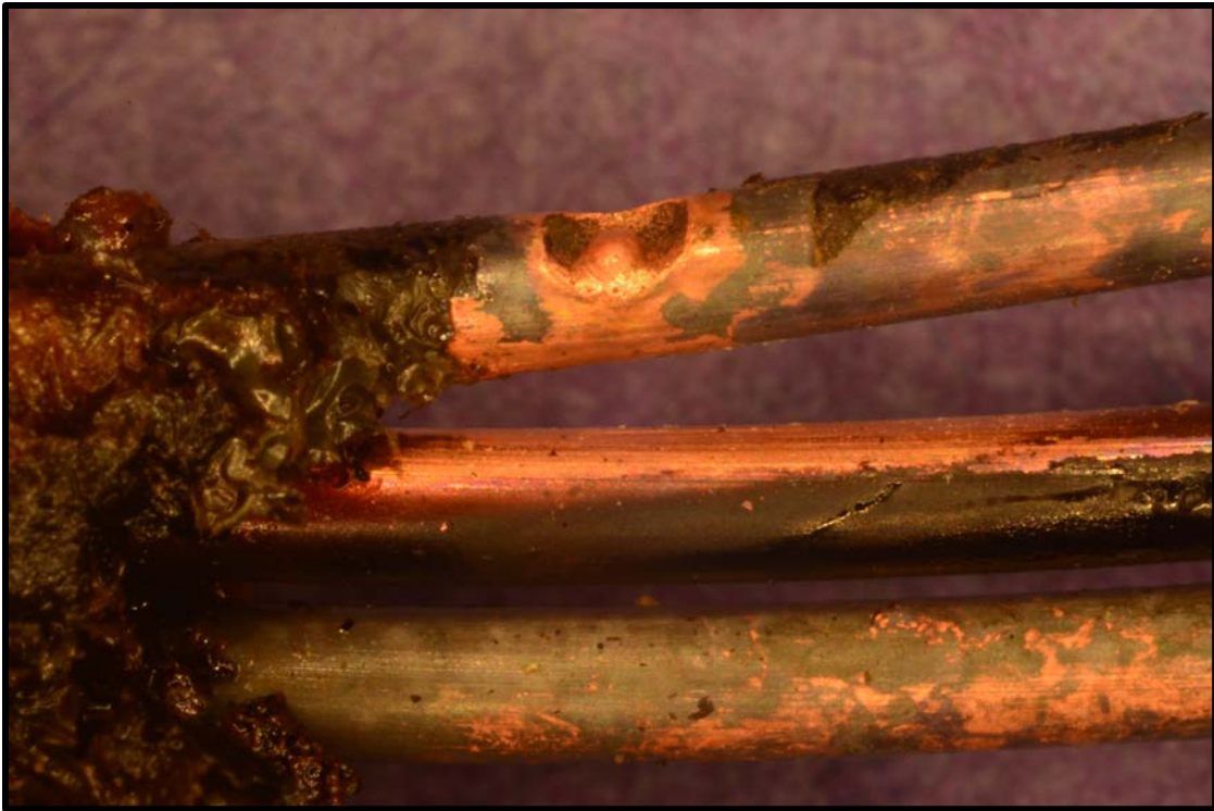
Figure 27. Arc melting produced during Test 4 of a GFCI circuit breaker at 35 kW/m 2 .
