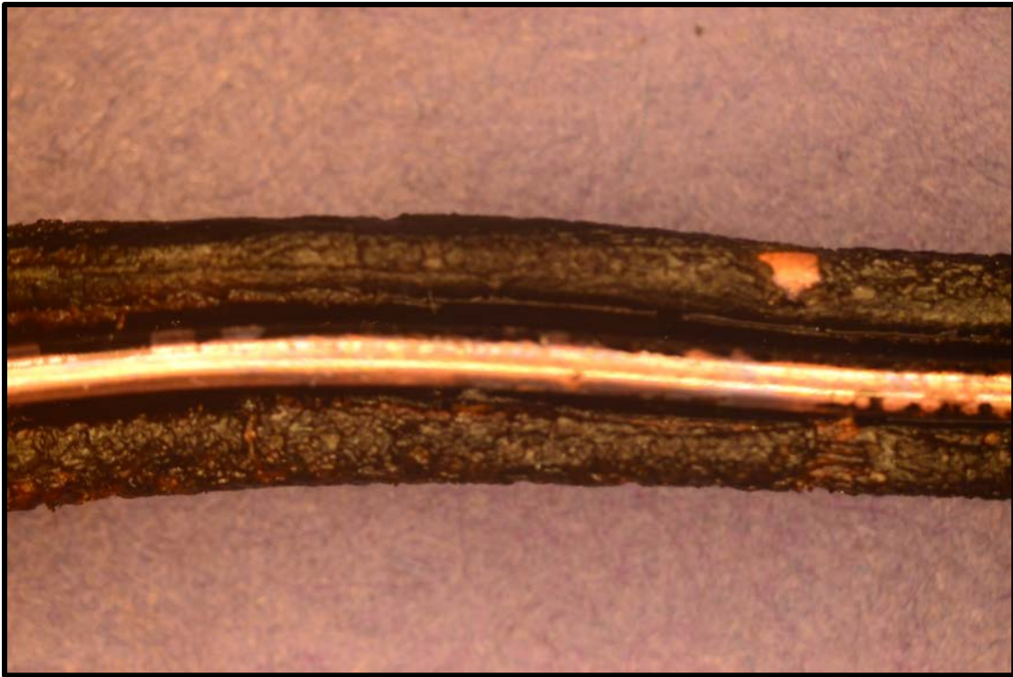
Figure 31. Absence of arc melting produced during Test 2 of a GFCI circuit breaker at 45 \text{ kW/m}^2 .
