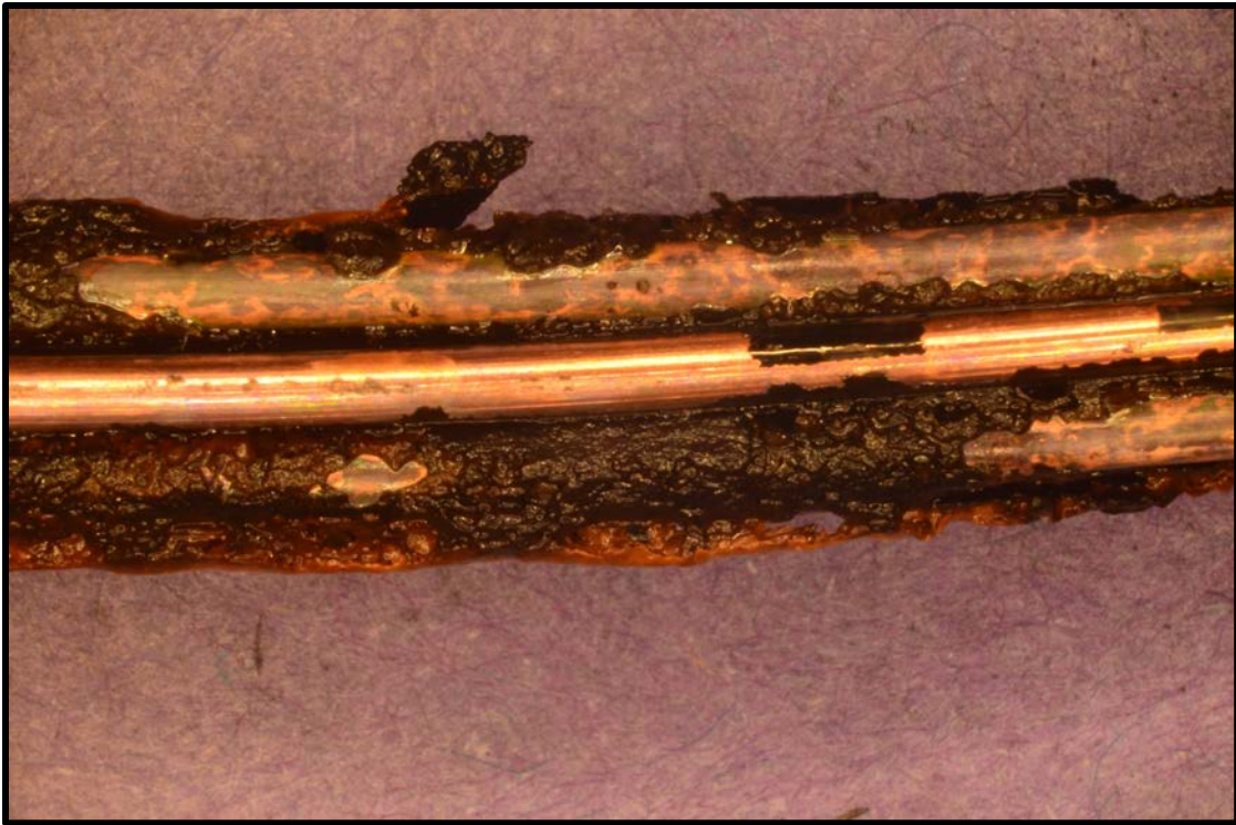
Figure 21. Absence of arc melting produced during Test 1 of a GFCI circuit breaker at 35 kW/m 2 .
