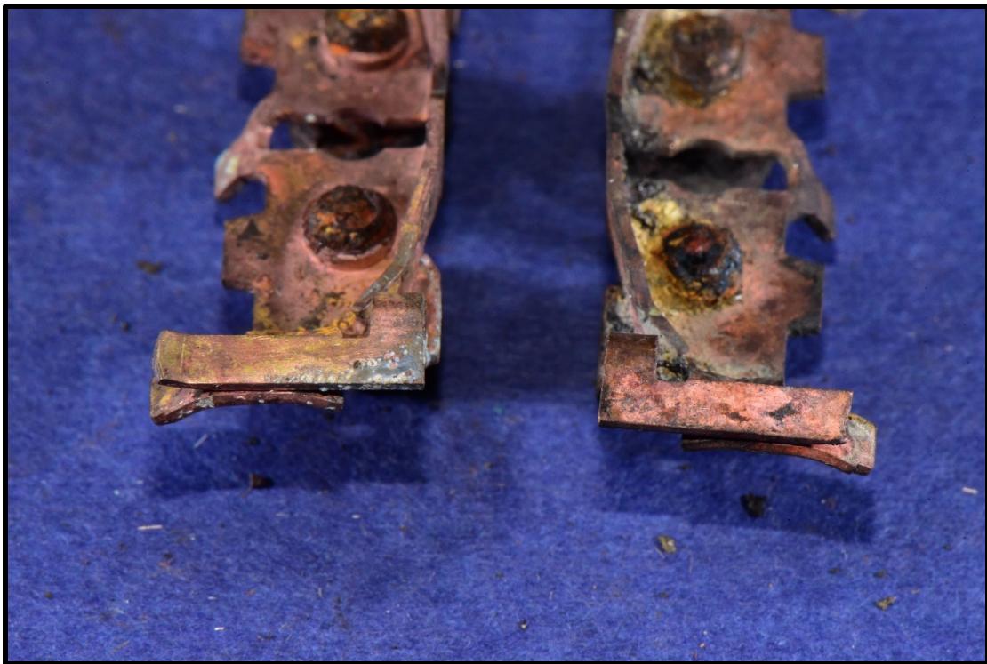
Figure 16. Bottom blade receptors from Receptacle 2-O
