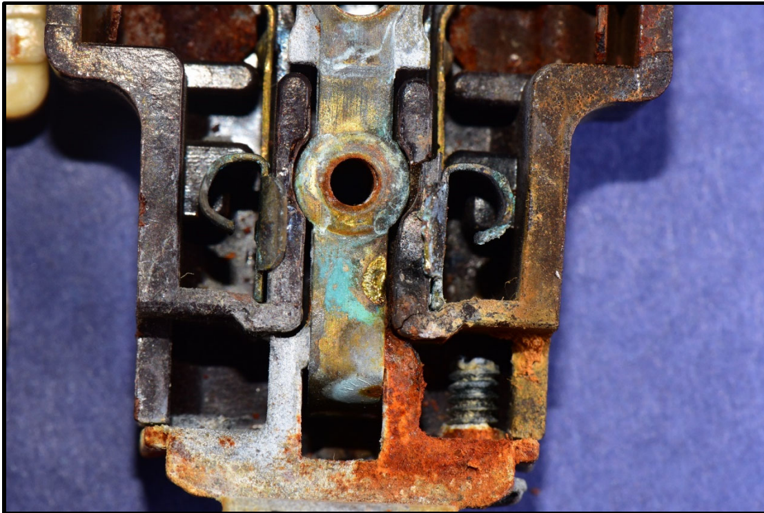
Figure 84. Power rails and ground yoke of Receptacle 23-T
