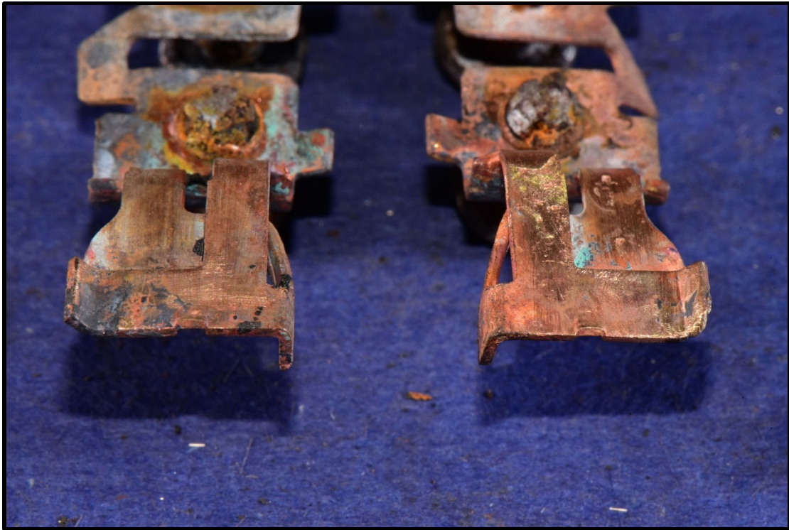
Figure 101. Bottom blade receptors from Receptacle 16-A
