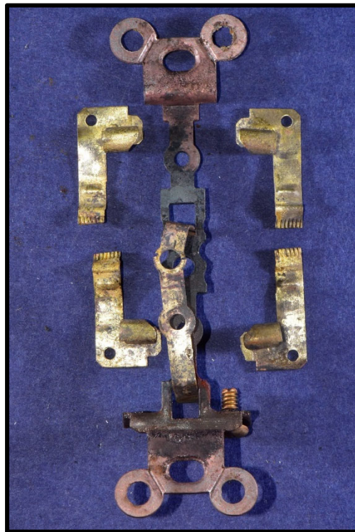
Figure 81. Power rails and ground yoke from Receptacle 23-T
