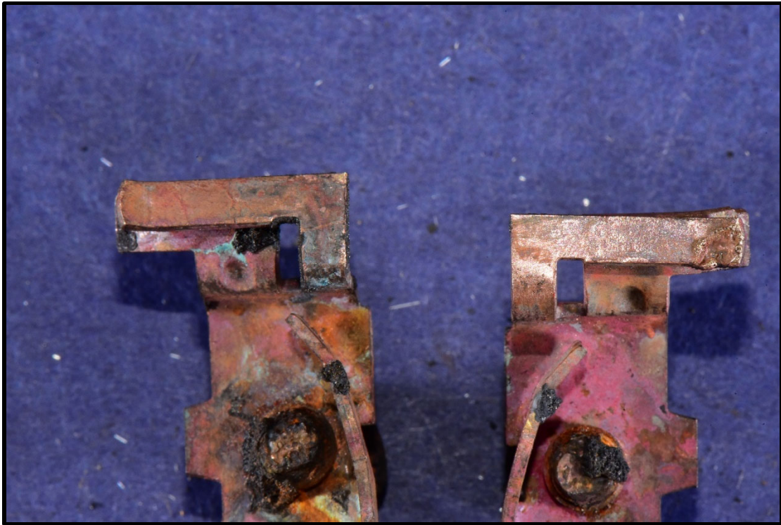
Figure 93. Top blade receptors from Receptacle 11-B
