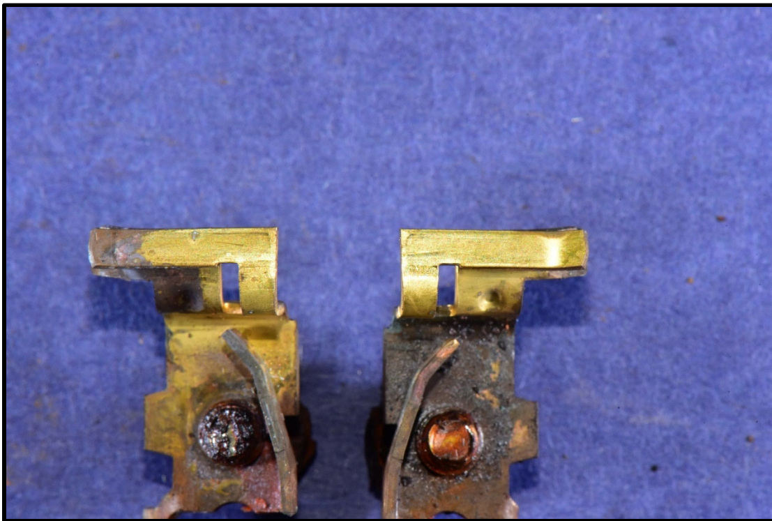
Figure 61. Top blade receptors from Receptacle 17-S
