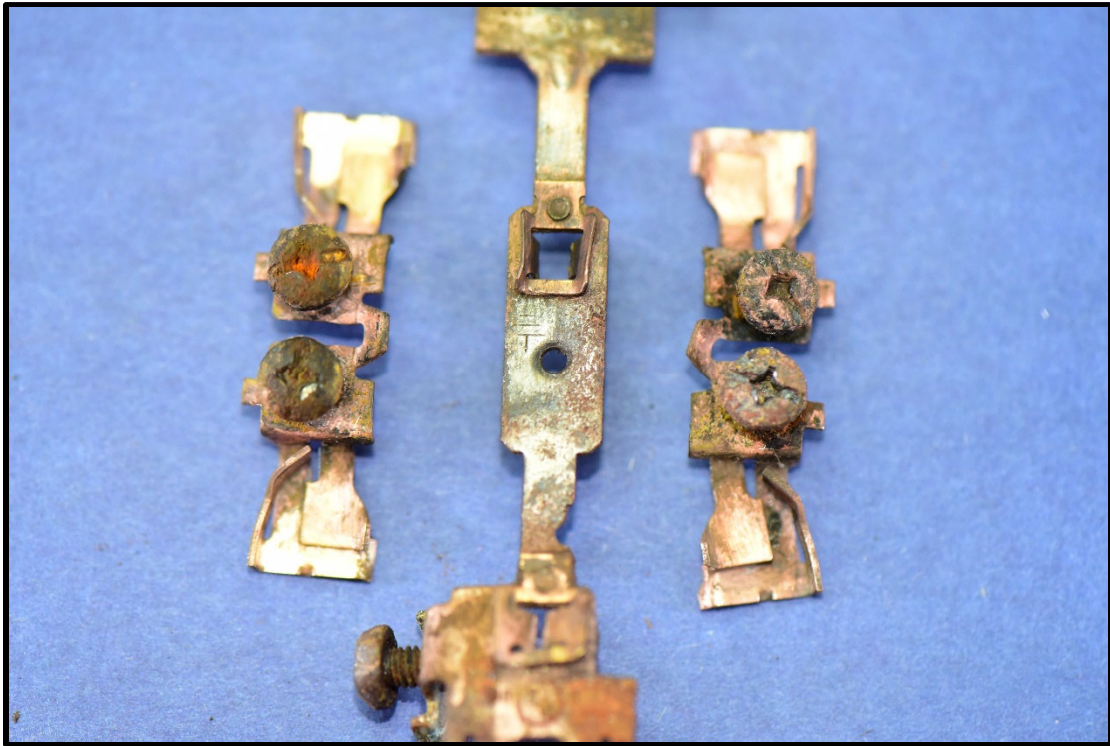
Figure 5. Receptacle I-T power rails and ground yoke
