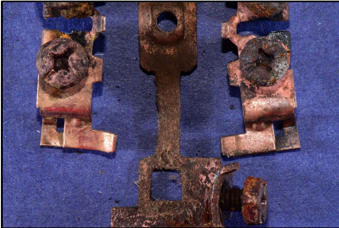
Figure 68. Power rails and ground yoke of Receptacle 17-T
