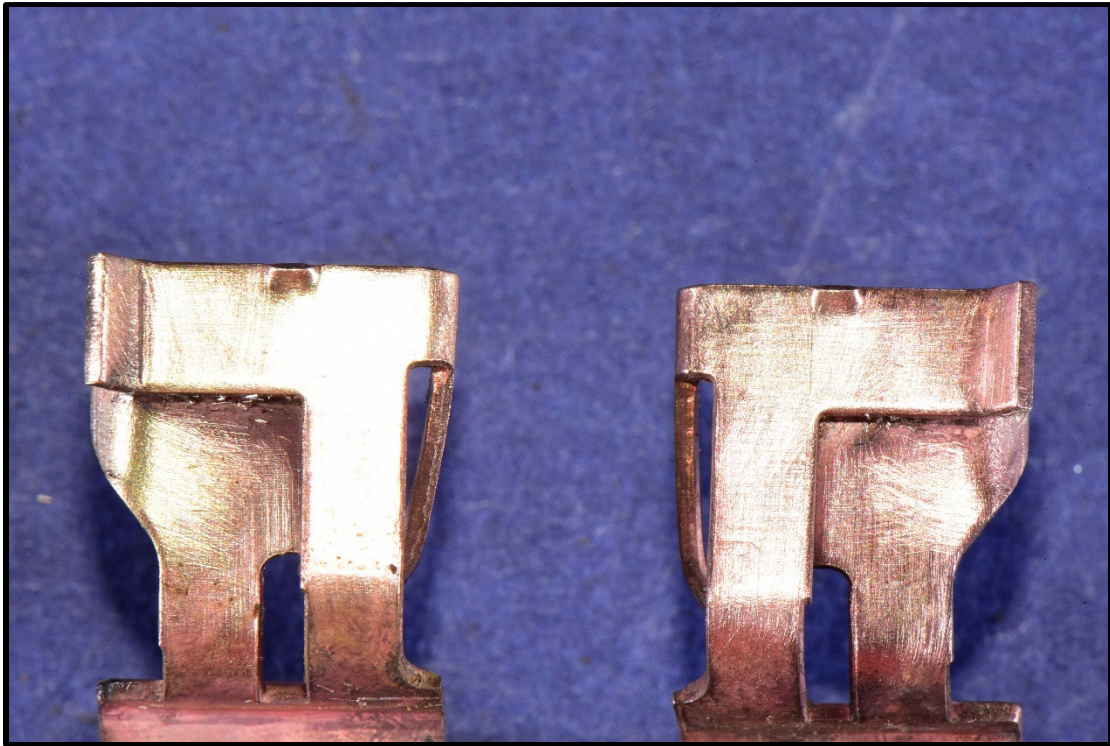
Figure 7. Top blade receptors for Receptacle 1-T
