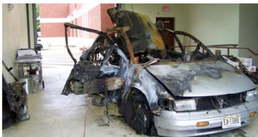
*On September 27, 2008, an ATF SACH team deploys to Cranbury New Jersey, to investigate a vehicle explosion (left). ATF K9 Ithaca alerts at numerous locations on the vehicle. Lab tests come back inconclusive for explosive residue. Suspect later states the cause of the explosion was 5 gallons of concentrated hydrogen peroxide on the vehicle's front seat. Photo by Special Agent/PIO Chris Bombardiere, Newark Field Division*
