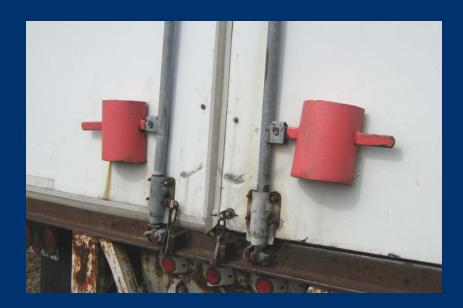
The locks above (from a common container/trailer) are not in compliance. The right door (looking at magazine) is only locked with one padlock.
