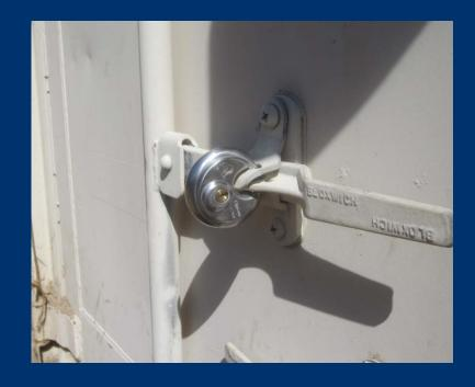
"Shrouded" padlocks (left) and disc padlocks (right) do not prevent the sawing or lever action on the locks, hasps or staples. Therefore, they must be protected with ¼-inch steel hoods
