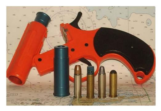
FTB personnel conducted testing using four flare launchers provided by Orion. The purpose of this testing was to determine the efficacy of certain adapters which allow the use of conventional ammunition in the Orion flare launchers. Orion submitted two each of their 12 Gauge and 25mm flare launchers:
