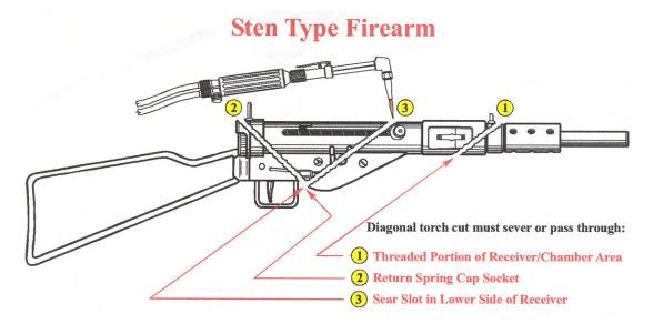
Alternative methods of destruction may also be acceptable. These alternative methods must be equivalent in degree to the approved method of destruction. Receivers that are not sufficiently modified cannot be approved for importation. To ensure compliance with the law, it is recommended that the importer submit in writing the alternative method of destruction to the ATF Firearms Technology Branch (FTB) for review and approval prior to importation.
