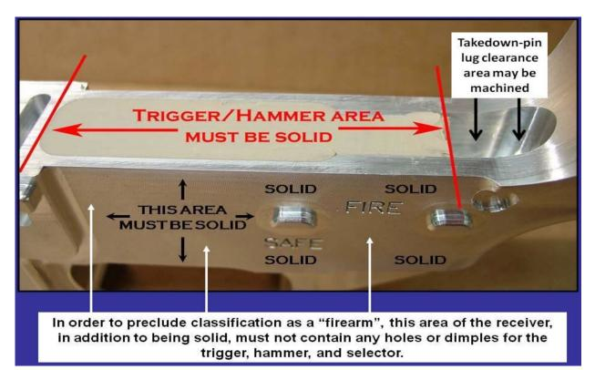
The following illustration demonstrates the fire control cavity of an AR-type receiver:
