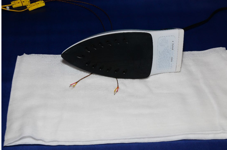
Figure 2. Placement of thermocouples. 51309_515188.jpg
