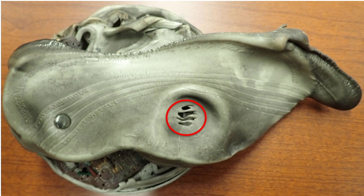
Figure 43. Example of an exposed smoke alarm without ESD on the external face of the horn chamber.
