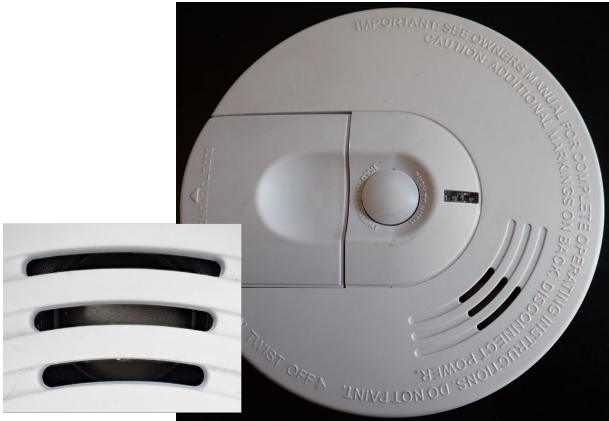
Figure 8. Example of a smoke alarm with insufficient, overall depositions of products of combustion. Note the lack of soot staining anywhere on the alarm.
