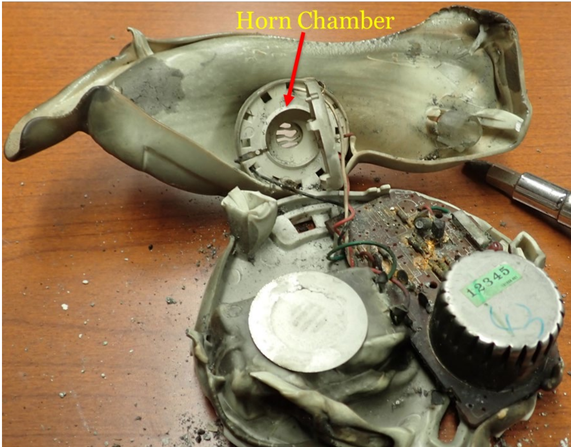
Figure 45. Example of an exposed smoke alarm without ESD within the horn chamber
