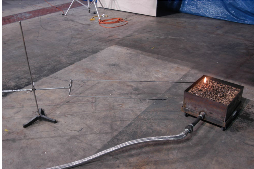
Figure 6. Propane “Wand” Ignition Source
