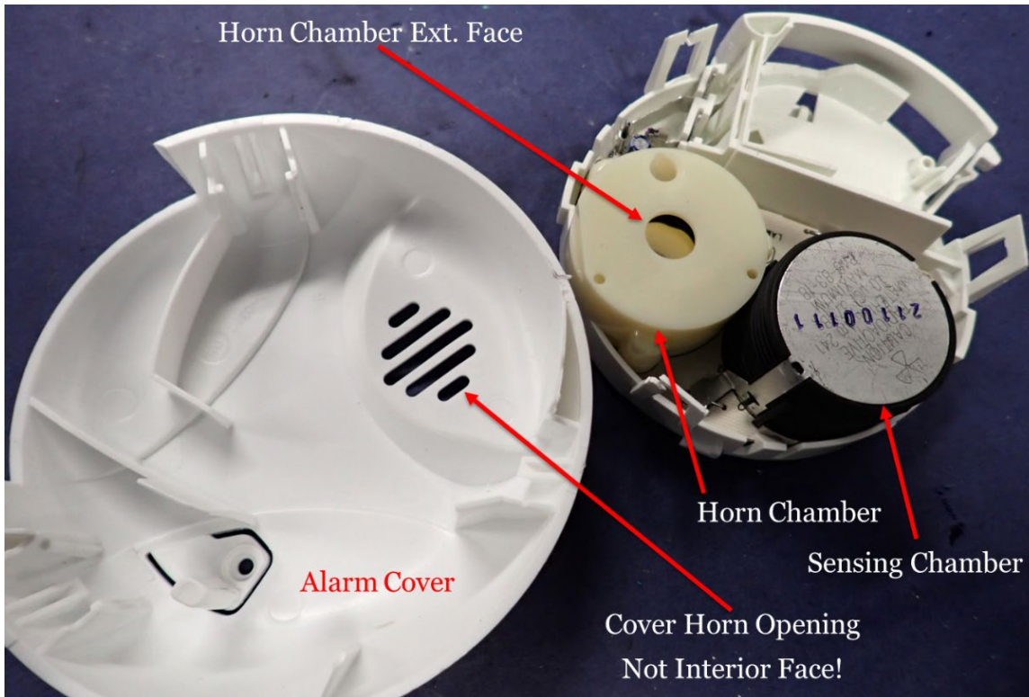
Figure 12. Example of a smoke alarm with internal horn chamber. Note how the horn chamber is not physically attached to the opening on the alarm cover.
