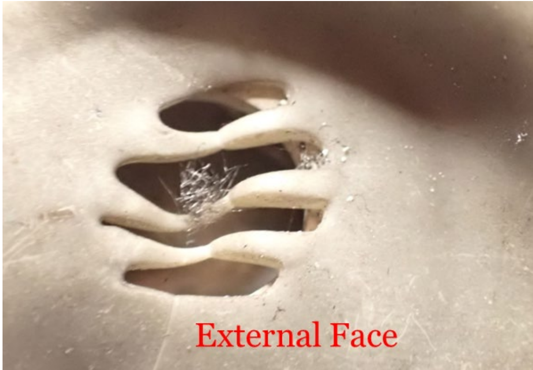
Figure 44. Example of an exposed smoke alarm without ESD on the external face of the horn chamber.
