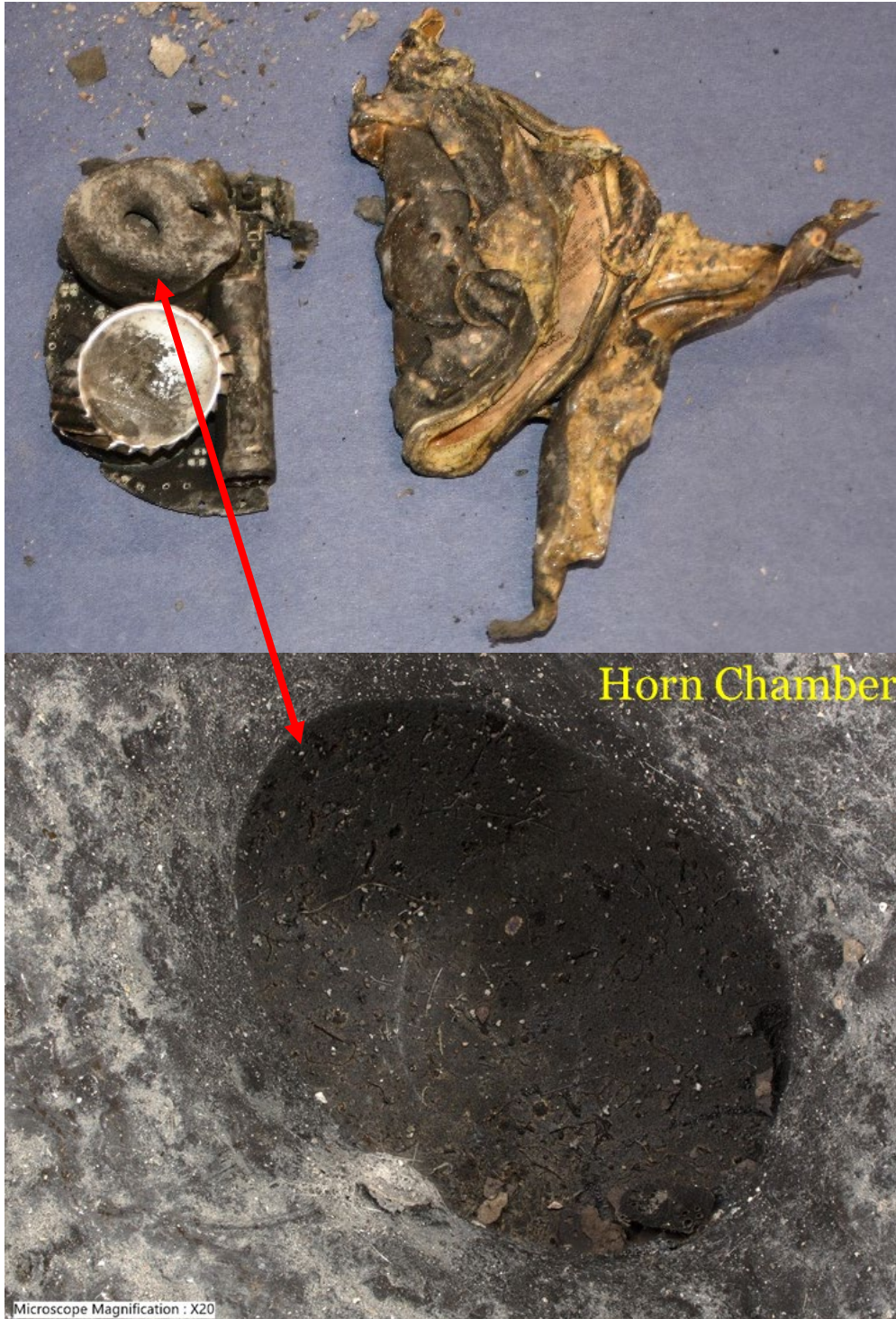
Figure 6. Example of a smoke alarm with thermal damage sufficient to alter observable indicators. Note the deformation and discoloration on the horn chamber.
