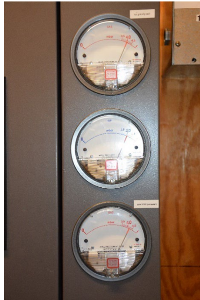
Figure 5. Combustion Calorimeter Pressure Gauges.
