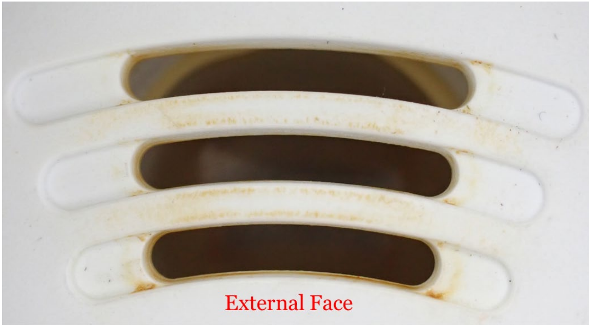
Figure 37. Example of a smoke alarm with ETD on the external face of the horn chamber.
