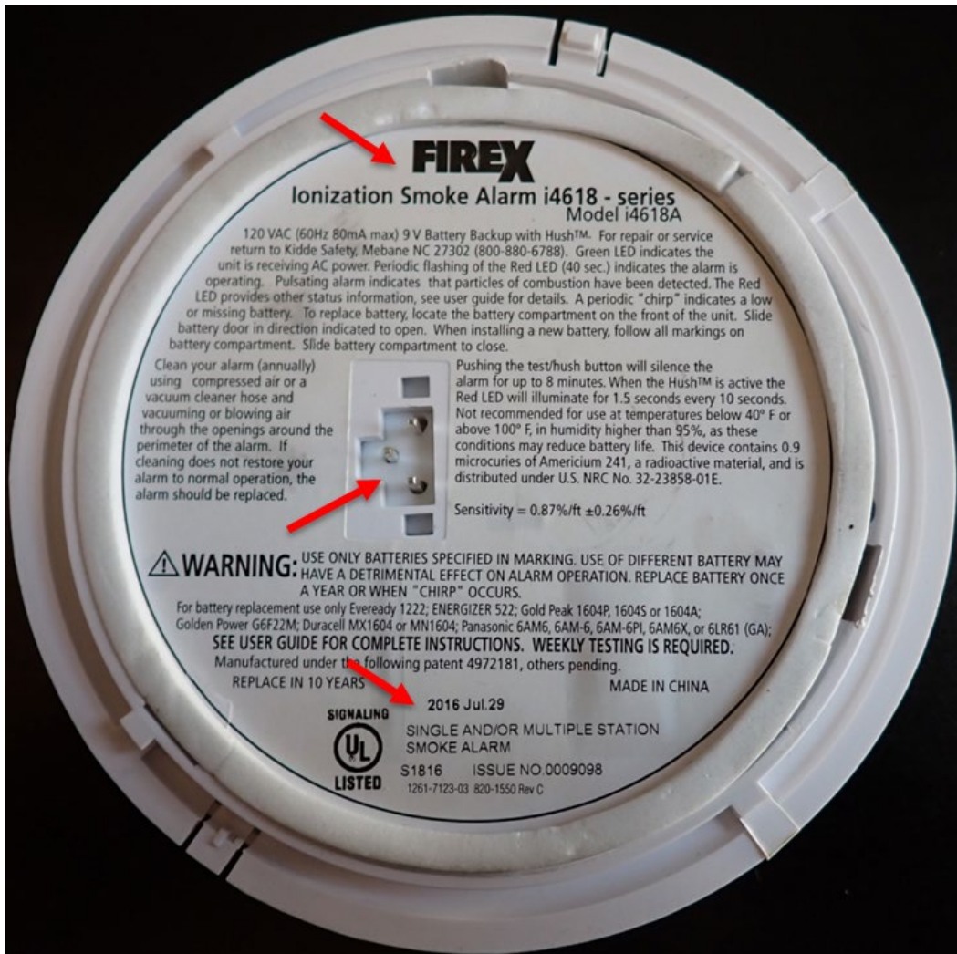
Figure 3. Example of alarm backside documentation. Note the Make/Model, Sensing Type, Manufacture Date, etc.
