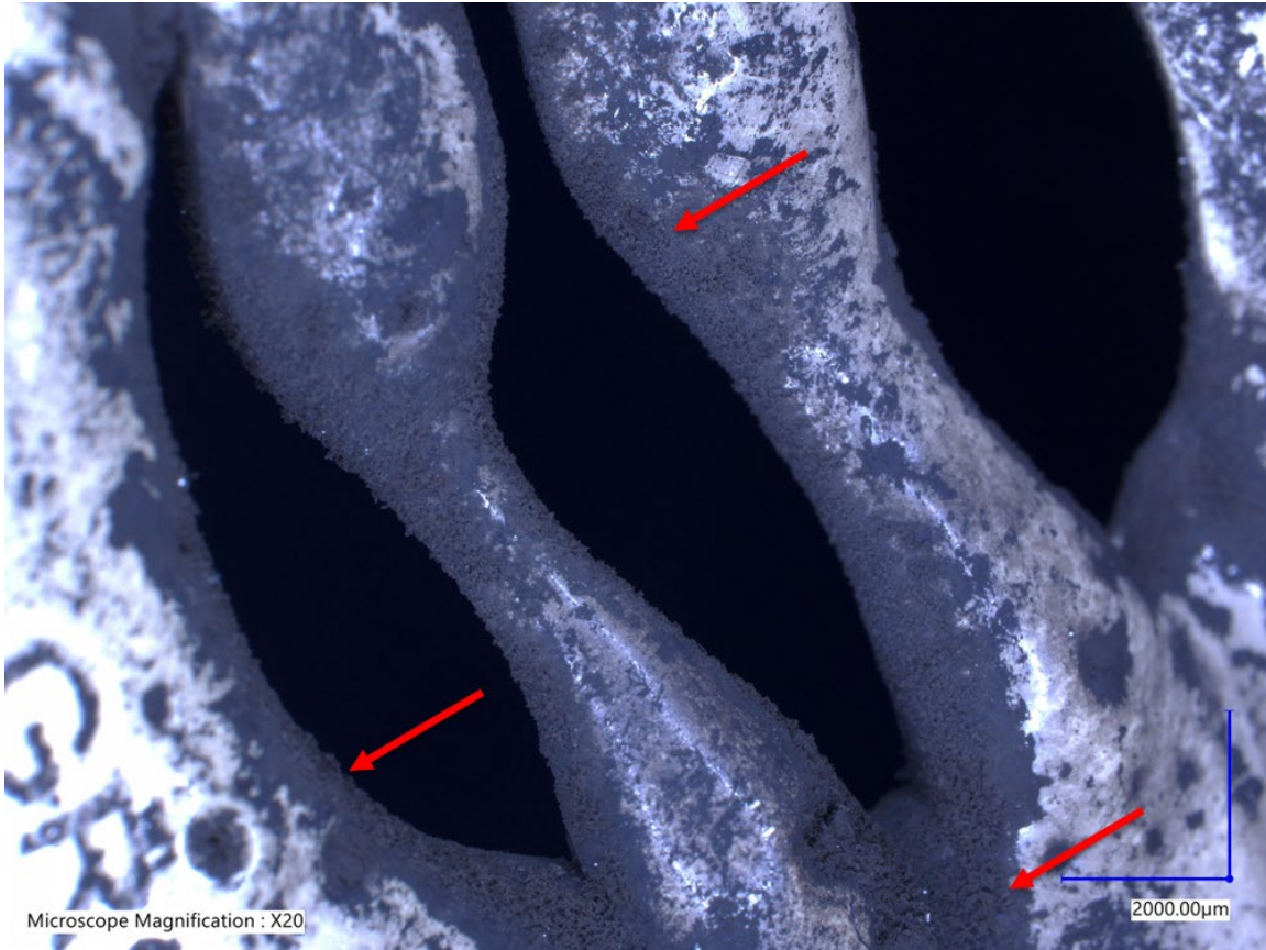
Figure 29. Example of a smoke alarm with ESD on the external and vertical faces of the alarm cover openings. Note the differential soot deposition, localized circumferentially around the openings in the alarm cover.
