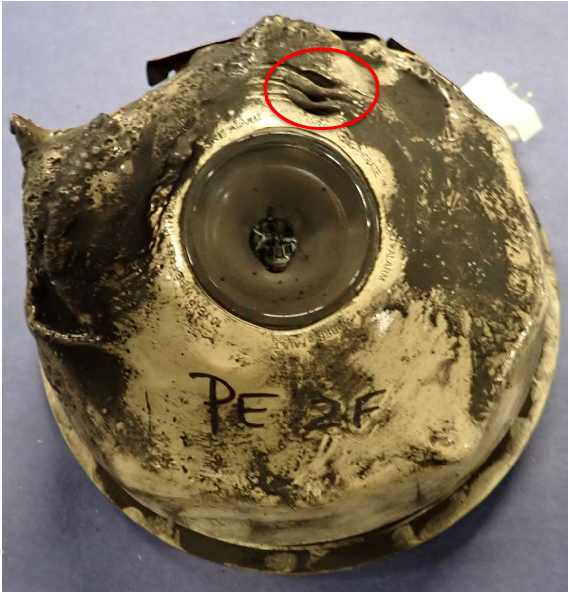
Figure 28. Example of alarm with horn chamber intimate with alarm cover.
