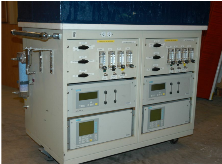
Figure 2. Cart housing of Siemens Oxymat 61 Analyzer
