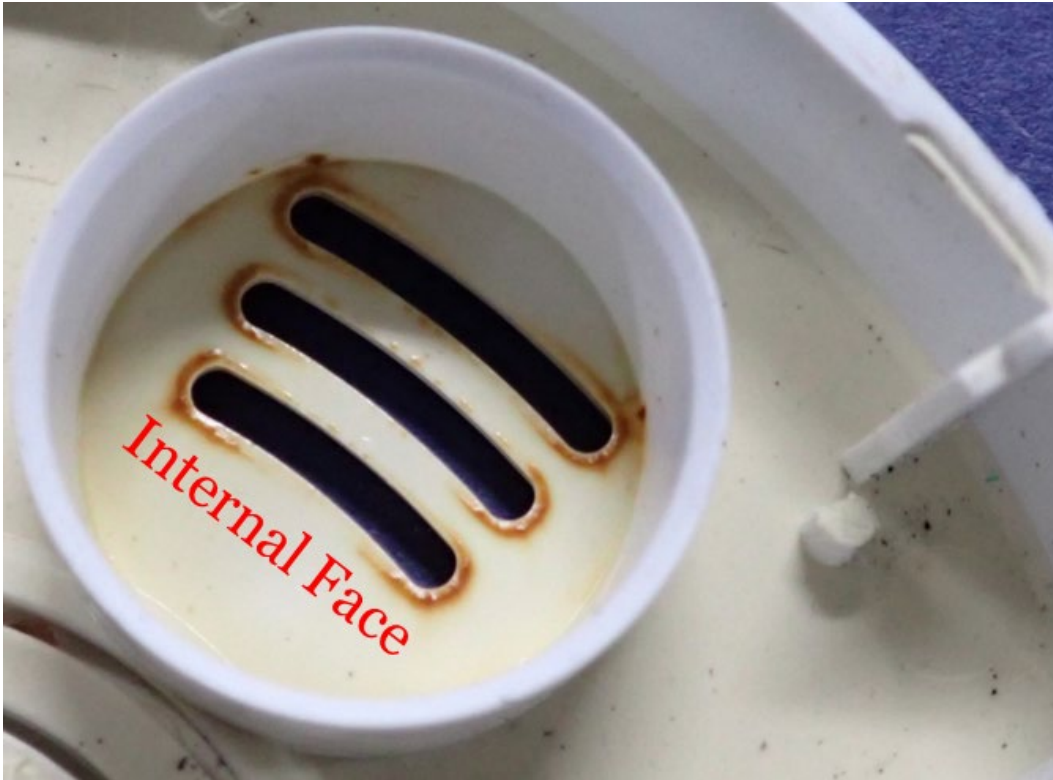
Figure 39. Example of a smoke alarm with ETD on the internal face of the horn chamber.
