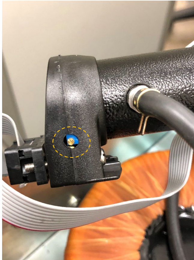
Figure A5. CO Cell Coarse Zero Potentiometer
