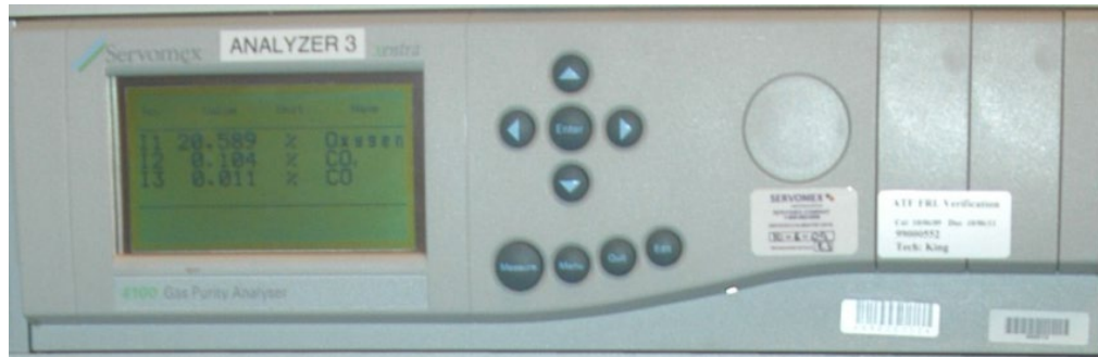
Figure 1: Servomex 4100 Gas Purity Analyzer
