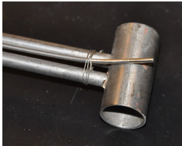
Figure 3: Shielded thermocouple mounted to a bi-directional probe
