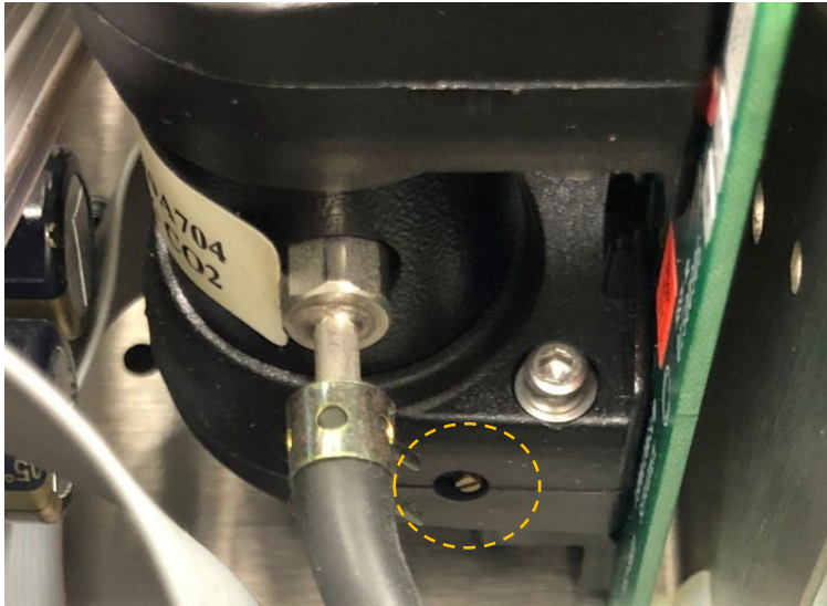
Figure A3. CO 2 Cell Coarse Zero Potentiometer
