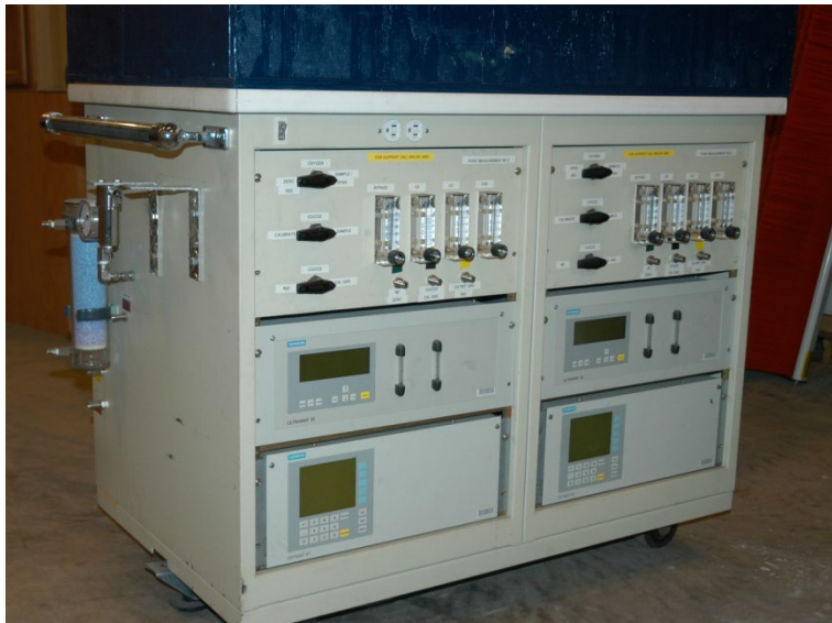
Figure 2. Cart housing of Siemens Ultramat 23 Analyzer
