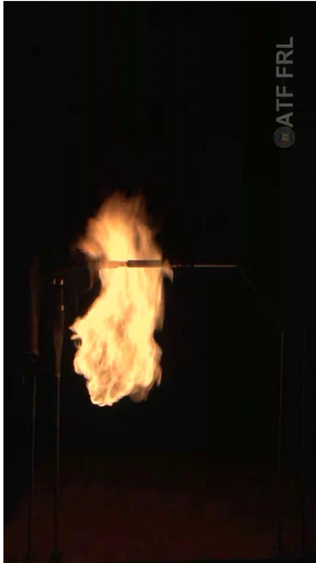
Figure 8. Resulting flame with the hole in the downward direction for Test 55 (still image obtained from video 348111_20210624_10.mov)
